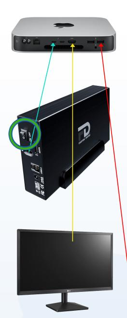
The Fantom hard drive(s) will connect to the server with the cable that came in the package (USB-B to USB-C cable) (Illustrated with the teal line). The drive needs external power, AND the power switch (Green circle) turned on to fully function.
