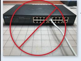
When connecting to the server or router use the uplink ports, not the standard PoE ports
