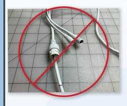
Use the caps to prevent moisture from entering the camera and network connection.
