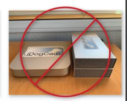
Stacking the drives causes heat to build up and shorten the life of the drives.
