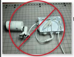
Use the rubber grommets to prevent bugs and rodents from nesting in the box. This also keeps the cables from sliding out.
